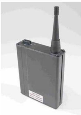
CaReader collects data from up to 8,000 meters. When required, it provides two-way communication with the TransMeter for programming and change of parameters.
